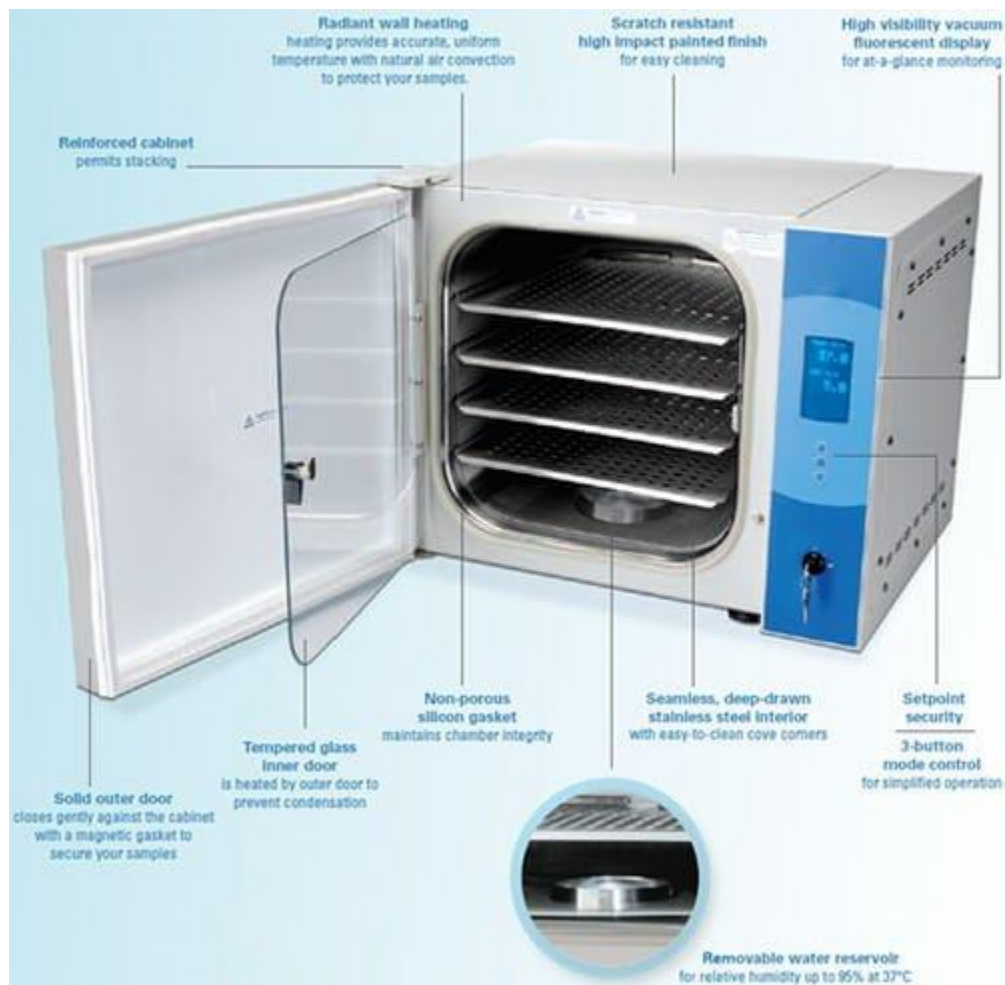
Figure 1: incubator components.
