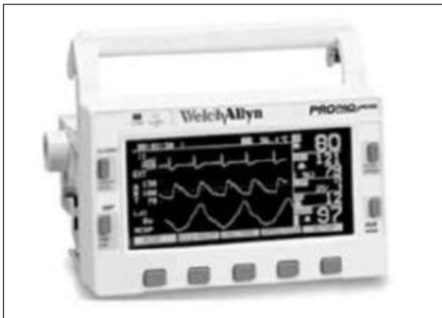
Figure 2: Vital signs monitor (Courtesy: M/s Welch Allyn)
