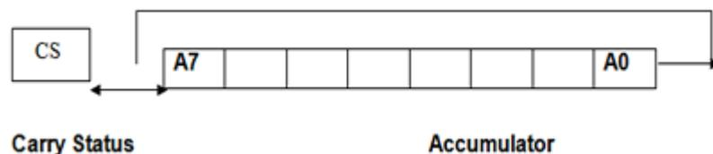
The content of the accumulator is rotated right by one bit. The zero bit of the accumulator is moved to the seventh bit as well as to carry bit. Only CS flag is affected.
