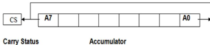
The content of the accumulator is rotated left by one bit. The seventh bit of the accumulator is moved to carry bit as well as to the zero bit of the accumulator. Only CS flag is affected.
